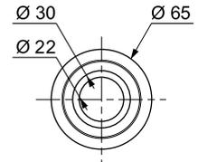
M47 Joint de clapet MPMP 25 x 65 x 4
