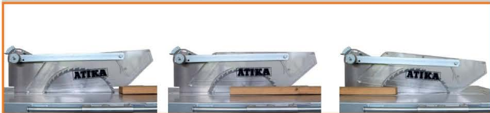
Transparent saw blade protective cover, which goes with the cut
